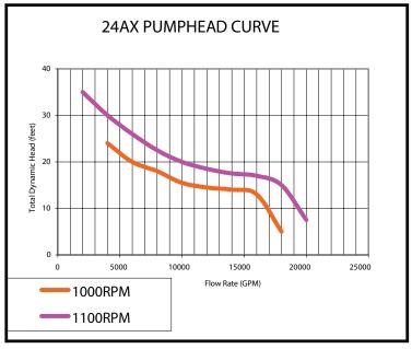
NOTE: SPEED IS BASED ON IMPELLER RPM.
