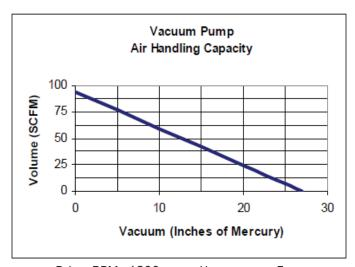
Driver RPM: 1800 Driven RPM: 850
