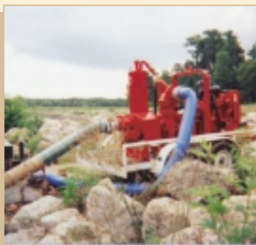
8NCRD 8" Non-Clog Pump used for a dewatering operation at Lake Kingwood in Kingwood, Texas.
