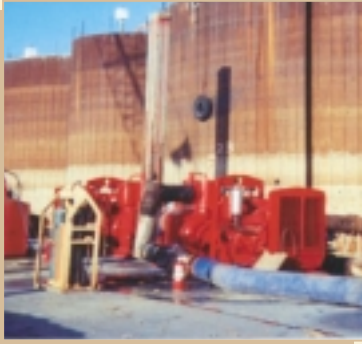
16NCRD 16" Non-Clog Pump used for a project at the Olmstead Lock & Dam in Olmstead Illinois
